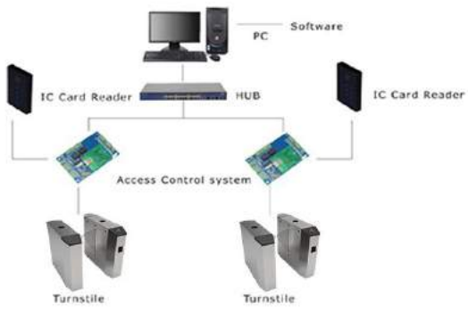
Access Control System
